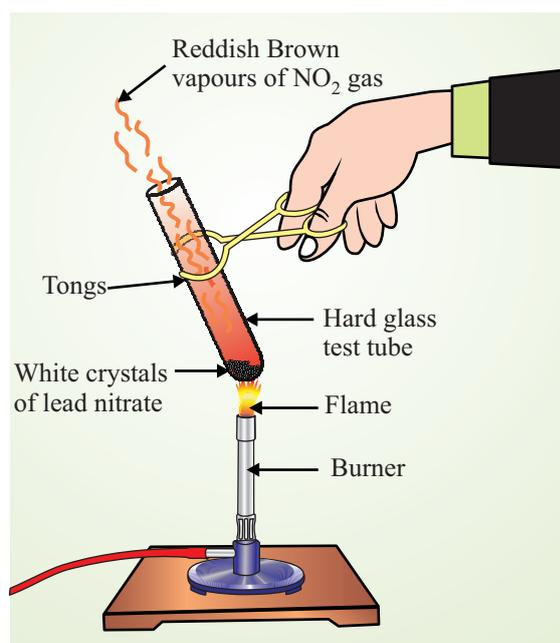
**Fig. 20.2** *Heating of lead nitrate*
