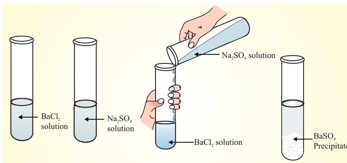
**Fig. 20.4** Double displacement reaction between  $BaCl_2$  and  $Na_2SO_4$
