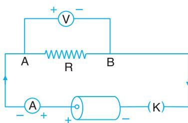
**Fig. 8.2 (a)** Circuit Diagram with single cell
