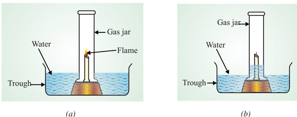
**Fig. 16.1** : Showing presence of oxygen in air(a) Before (b) After
