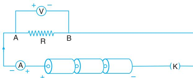
**Fig. 8.2 (c)** Circuit Diagram with three cells
