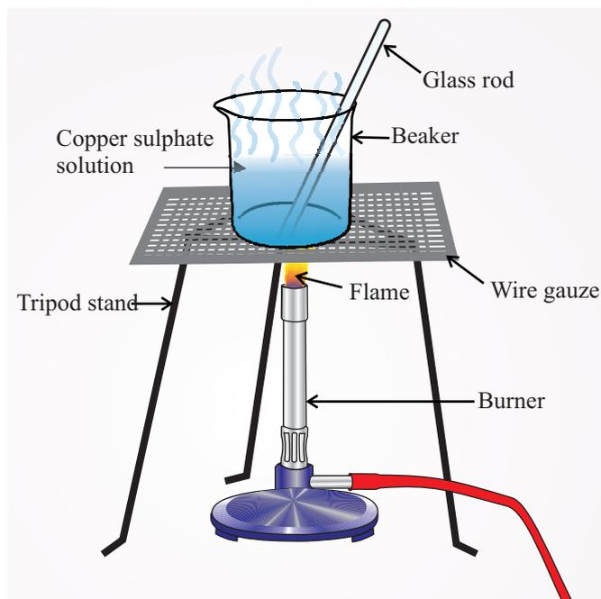
**Fig. 12.2 :** Concentration of the solution by heating
