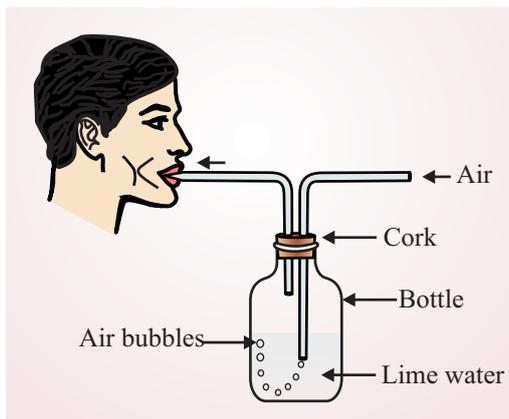
**Fig. 15.1 :** Testing presence of  $CO_2$  in air
