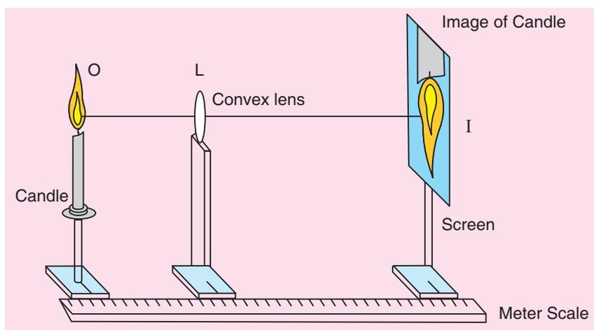
**Fig. 7.1:** Setting of the experiment for convex lens.
