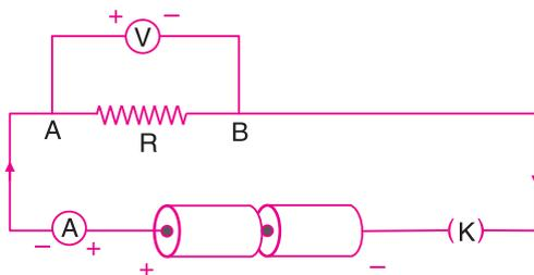
**Fig. 8.2 (b)** Circuit Diagram with two cells
