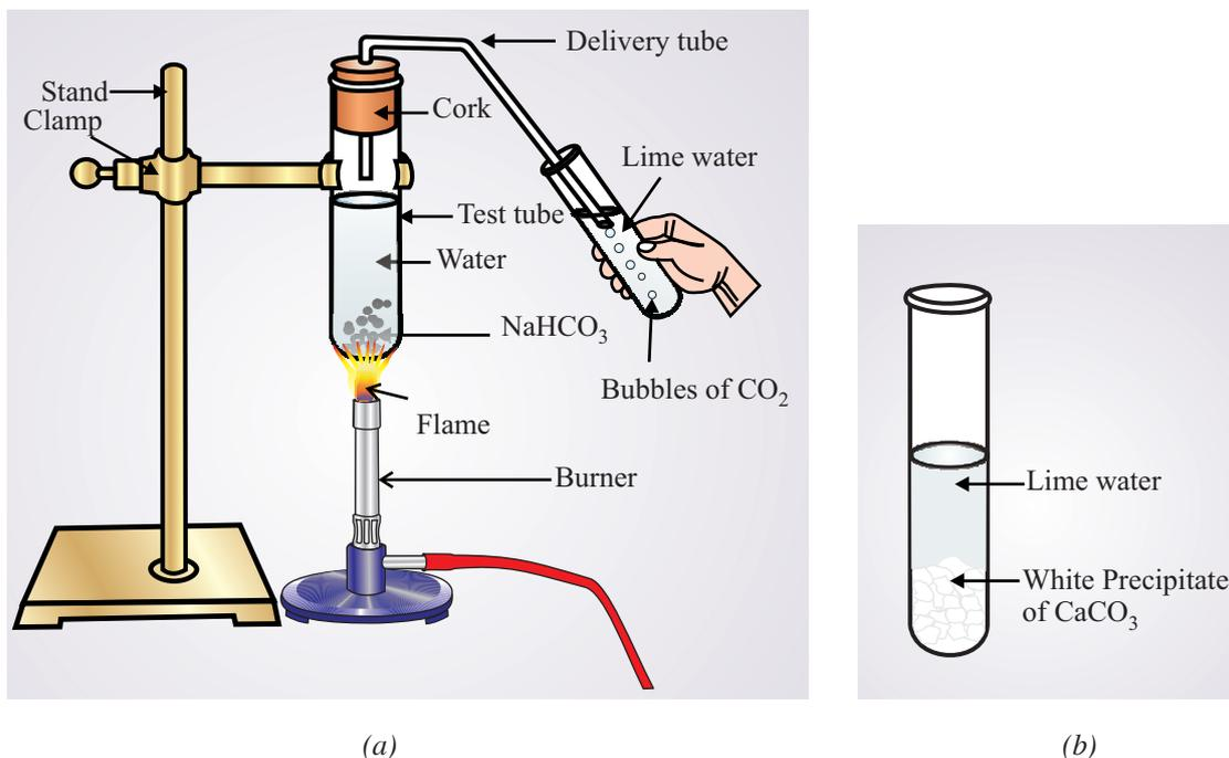
**Fig. 19.1:** (a) Heating of baking soda and passing the  $\text{CO}_2$  produced through lime water
