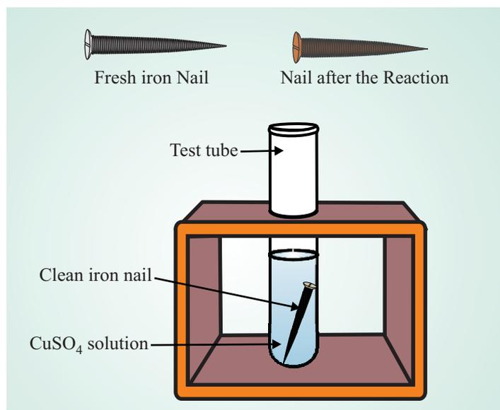
**Fig. 20.3** Displacement reaction between iron and  $\text{CuSO}_4$  Solution
