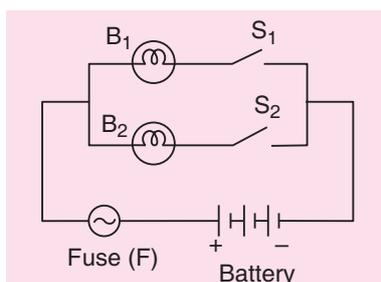
**Fig. 9.1** Circuit diagram for household circuit
